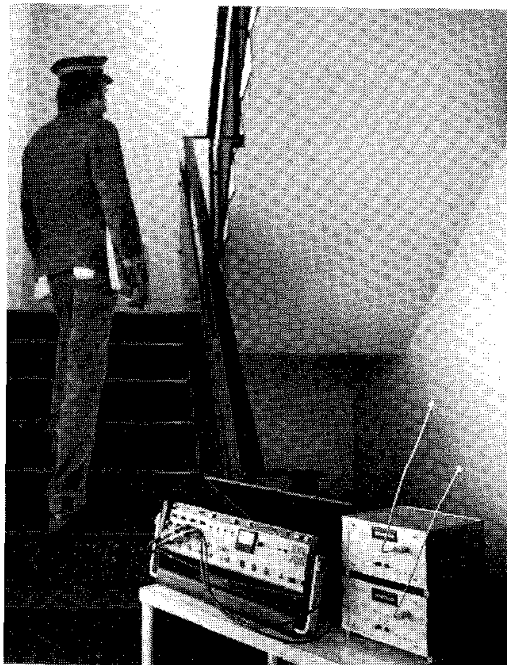
Fig. 3. Telemetry transmitters were employed in the study to relay the EMG from the back muscles to a tape recorder for later analysis.
